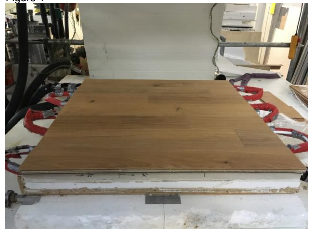
Multi-layer parquet installed on a test panel (floating installation)
