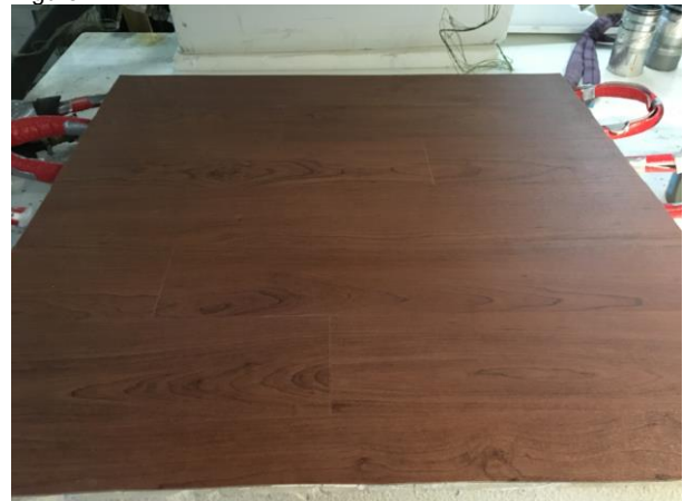
Vinyl flooring installed on a test panel (bonded installation)
