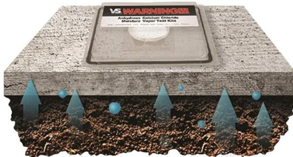
Calcium Chloride Test ASTM F1869-22
